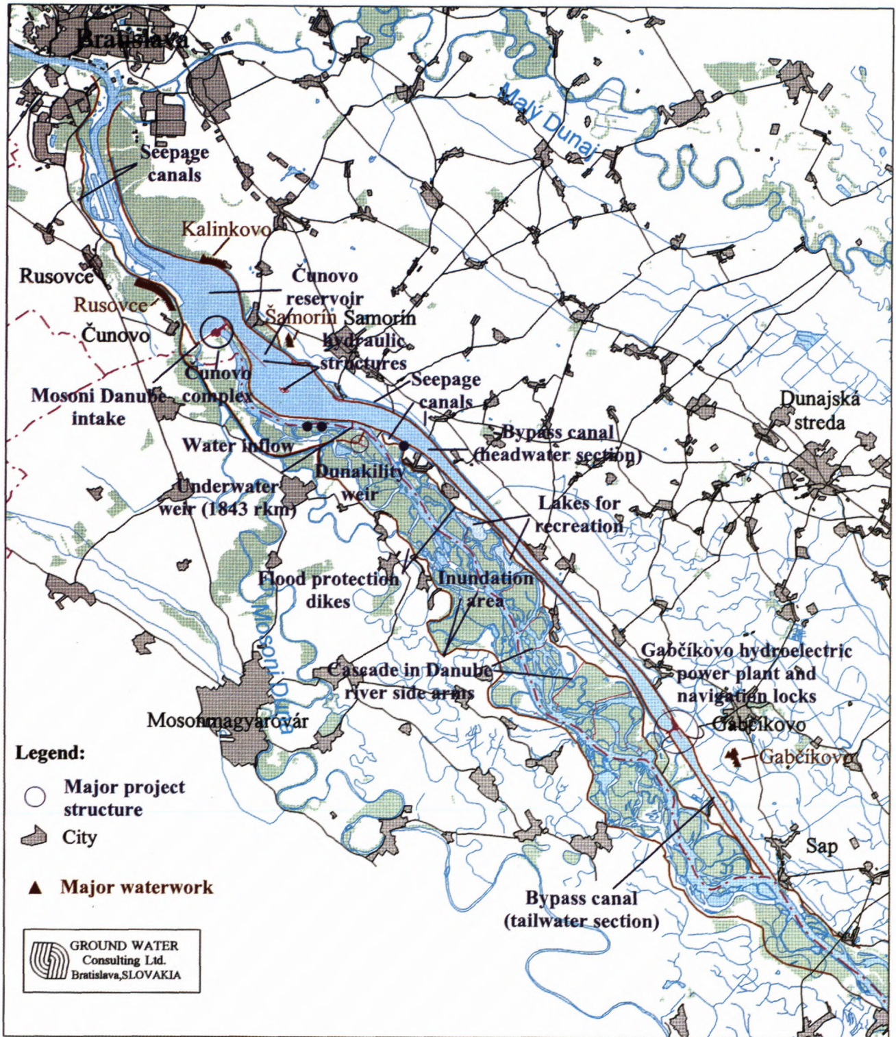
Fig. 1. Gabčíkovo part of the Project, technical means for managing surface and ground water regime.
